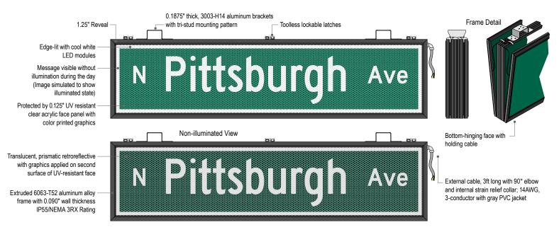
Outdoor full face signs with an aluminum cabinet, edge-lit with cool white LED modules. The sign message is formed by a translucent printed face with a prismatic retroreflective sheeting applied that illuminates when activated and remains viewable when deactivated
