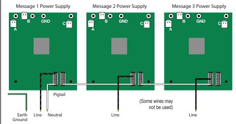
Each sign will have at least one power supply mounted to the back of the LED display board; this is where your connections will be made.
